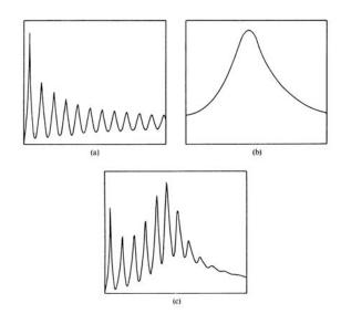
and; (graph c) mouthpiece and tube together. The frequency scale is horizontal from 0 to 1000 Hz. In graph (a) the resonances of the tube at 85 Hz and its harmonics are well recognizable. Graph (b) shows the broad resonance of the mouthpiece with a maximum at about 450 Hz. In graph (c) it is shown that when the mouthpiece is fitted to the tube, the resonances of the tube stay unmistakable. But in particular at the high frequency side of the mouthpiece resonance, the peak heights tend to
