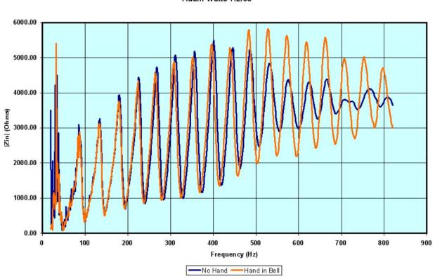
Conn 8D Open F-Side |Zin| Comparison for Hand Placement Adam Watts 7/2/09
