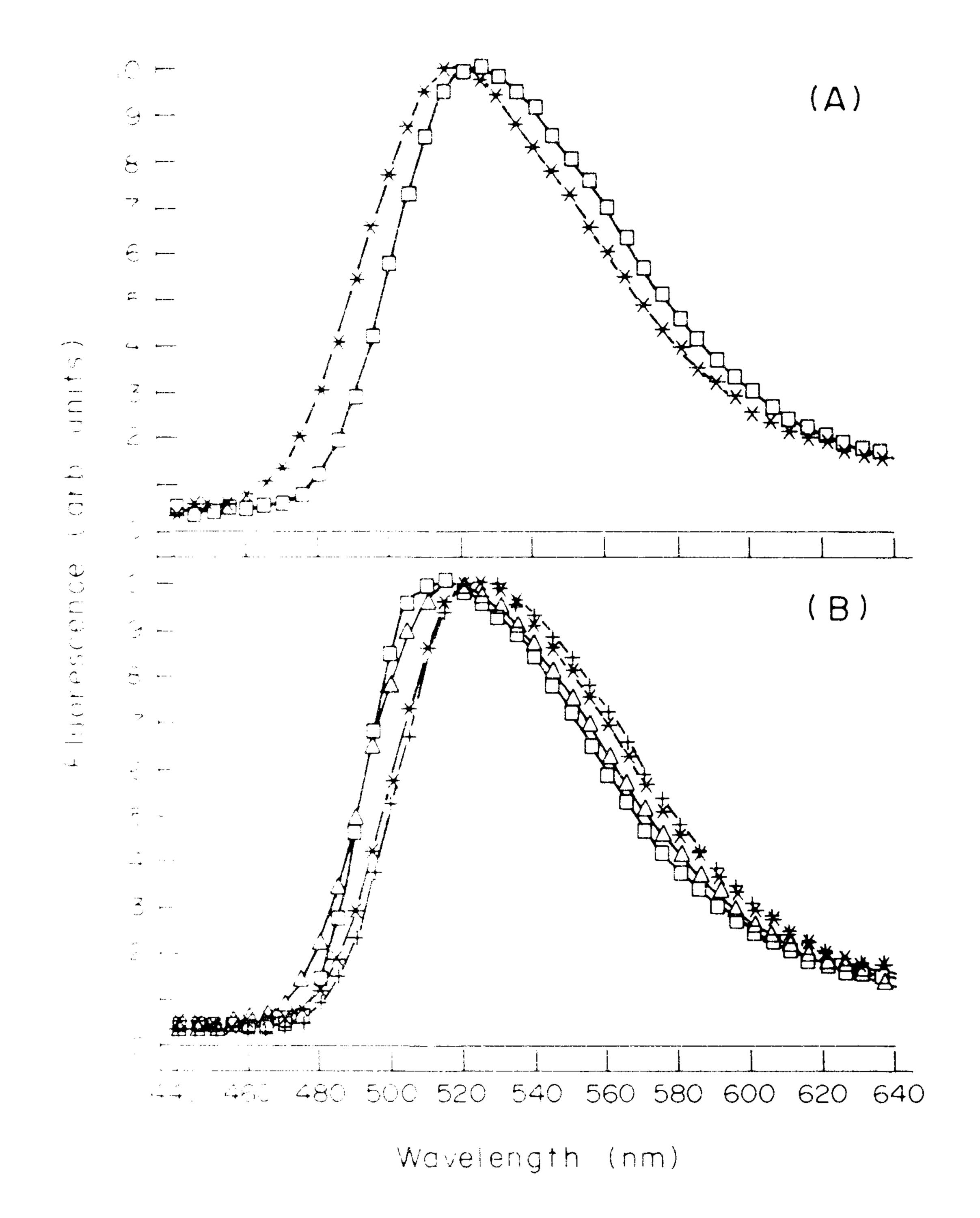
Figure 2. Peak normalized fluorescence spectra of FMN in surfactant entrapped water pools. (A) FMN in AOT, \*\*\*  $w_0 = 3.8$ . In DAP  $w_0 = 28.7$ . (B) FMN in water and in different micelles. The AOT  $w_0 = 28.7$ .  $\square \square \square w_0 = 4.9$ . CTAB  $w_0 = 9.4$ , +++ FMN in water. Further details as in the legend of Fig. 1.
